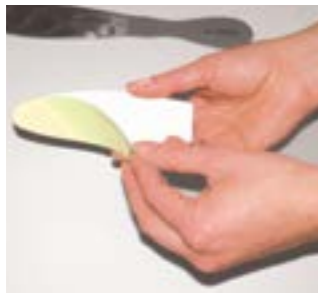
The fresh, self-adhesive surface is peeled from the carrier film.
